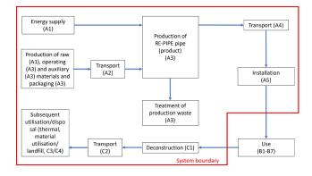
The following is a detailed list of the life cycle stages and process modules taken into account in the manufacture of the pipe:
